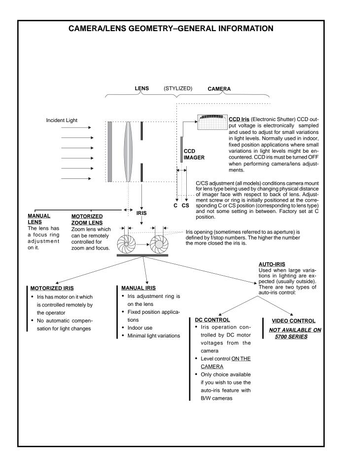
The purpose of backfocusing is to make the adjustments necessary for the picture to remain in focus throughout the camera's zoom range, which is the case for instance, in motorized zoom, auto iris configurations. Manual Iris lens/camera combinations also need to be backfocused. Follow the general instructions listed below to adjust backfocus appropriate to your camera/lens combination.
